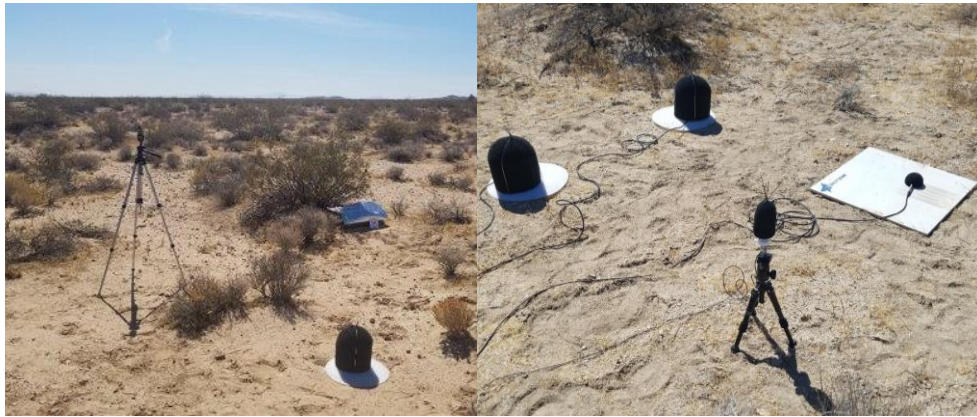
Figure 1. Example BYU Stations. Left: A base configuration station with data acquisition system (PUMA), tripod-mounted weather station, and COUGAR microphone configuration. Right: A microphone configuration comparison station with two COUGAR (left and top), one Elevated (bottom), and one Ground-Board configuration (right).
