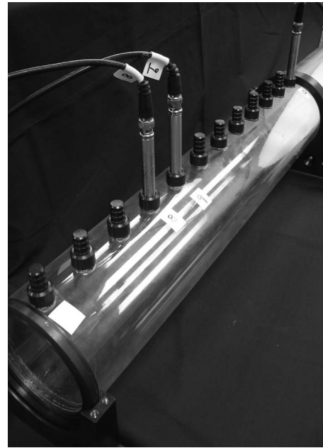
FIG. 5. Photograph of the receiving-side tube of the measurement system without a module attached. The microphone ports are spaced 5 cm apart and the tip of the anechoic wedge is visible near the end of the tube.
