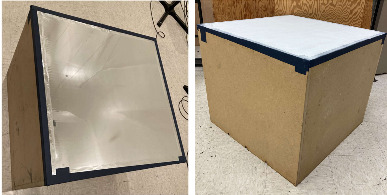
Figure 2. A visual of the enclosure used to simplify the problem. a) The mylar stretched across the MDF enclosure. b) A side view of the enclosure showing a developer spray used to make the mylar membrane easier to scan by the SLDV and the three ports drilled in the bottom left to feed the source cabling.
