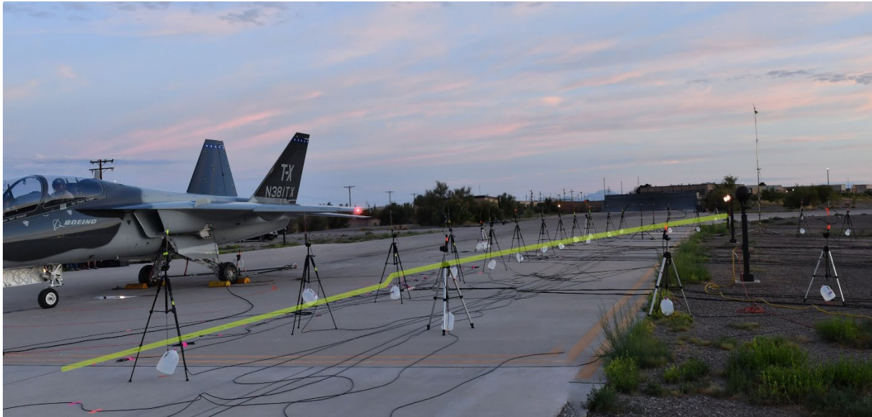
Figure 1. Photo of T-7A aircraft measurement with ground-based imaging array highlighted in yellow.
