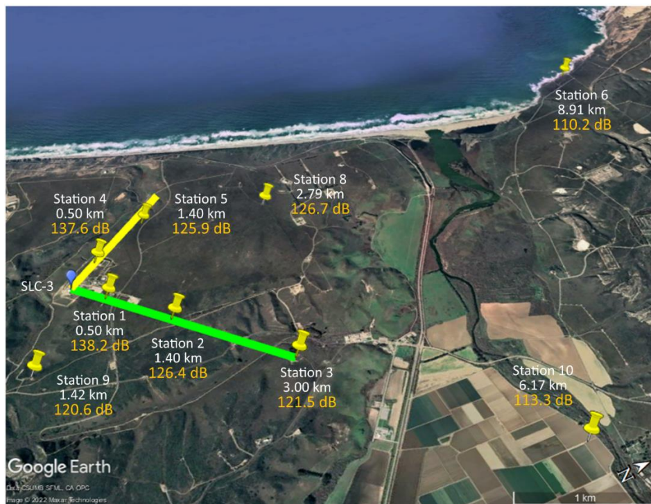
Figure 3: Locations of measurement stations with maximum OASPL values and distance from the launch site (SLC-3). The different radials are highlighted.
