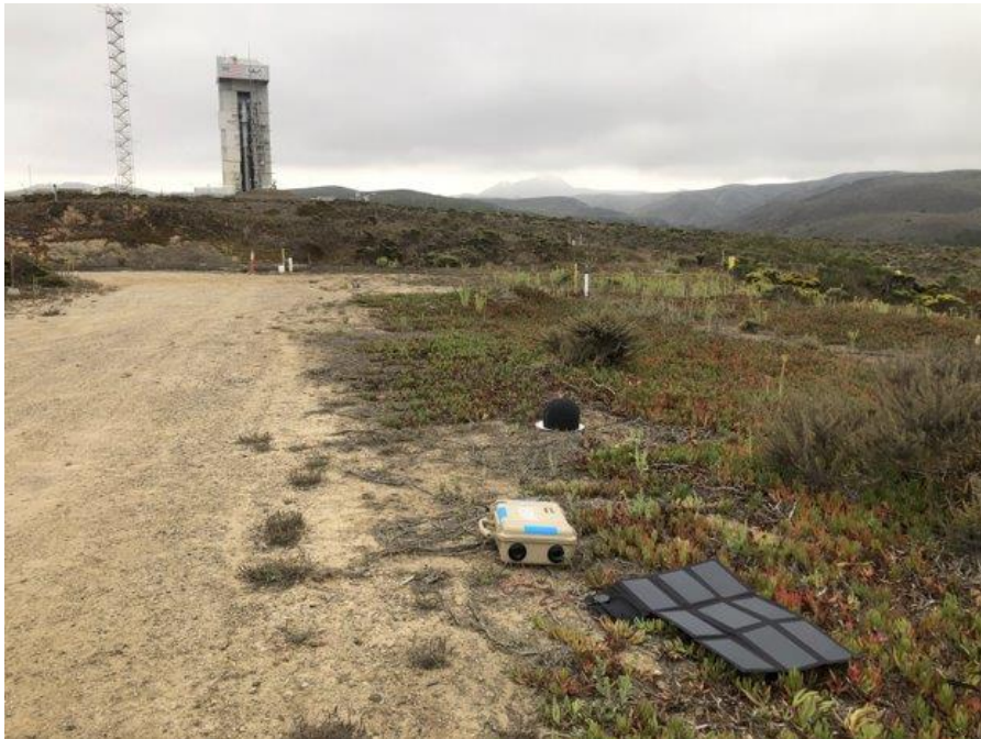
Figure 5: Example setup of Station 1. Included: a PUMA case(brown), COUGAR housing of the microphone shown by the black windscreen, and solar panel for independency.
