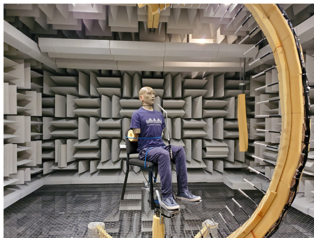
FIG. 10. (Color online) KEMAR HATS seated within a directivity measurement system.
