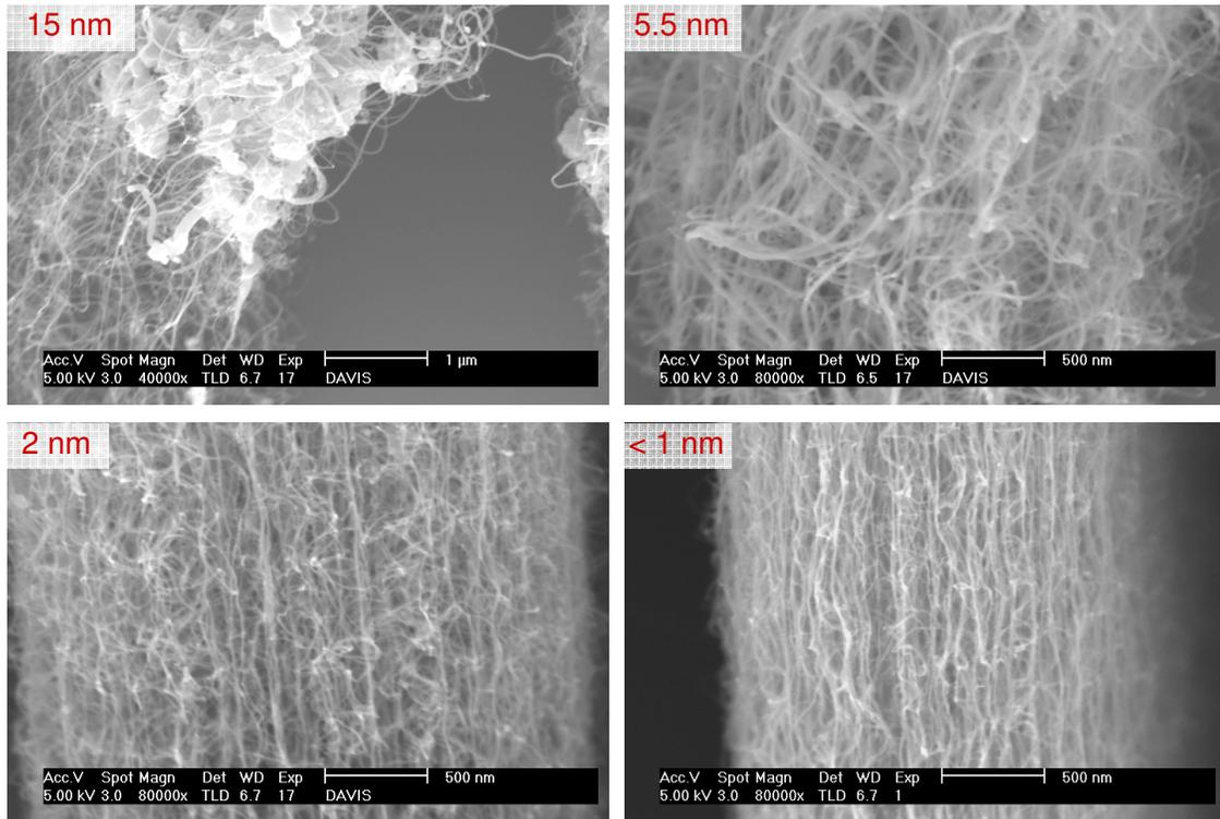
**Figure 3.4** SEM image of VACNT forest growth density with different Fe thickness'
