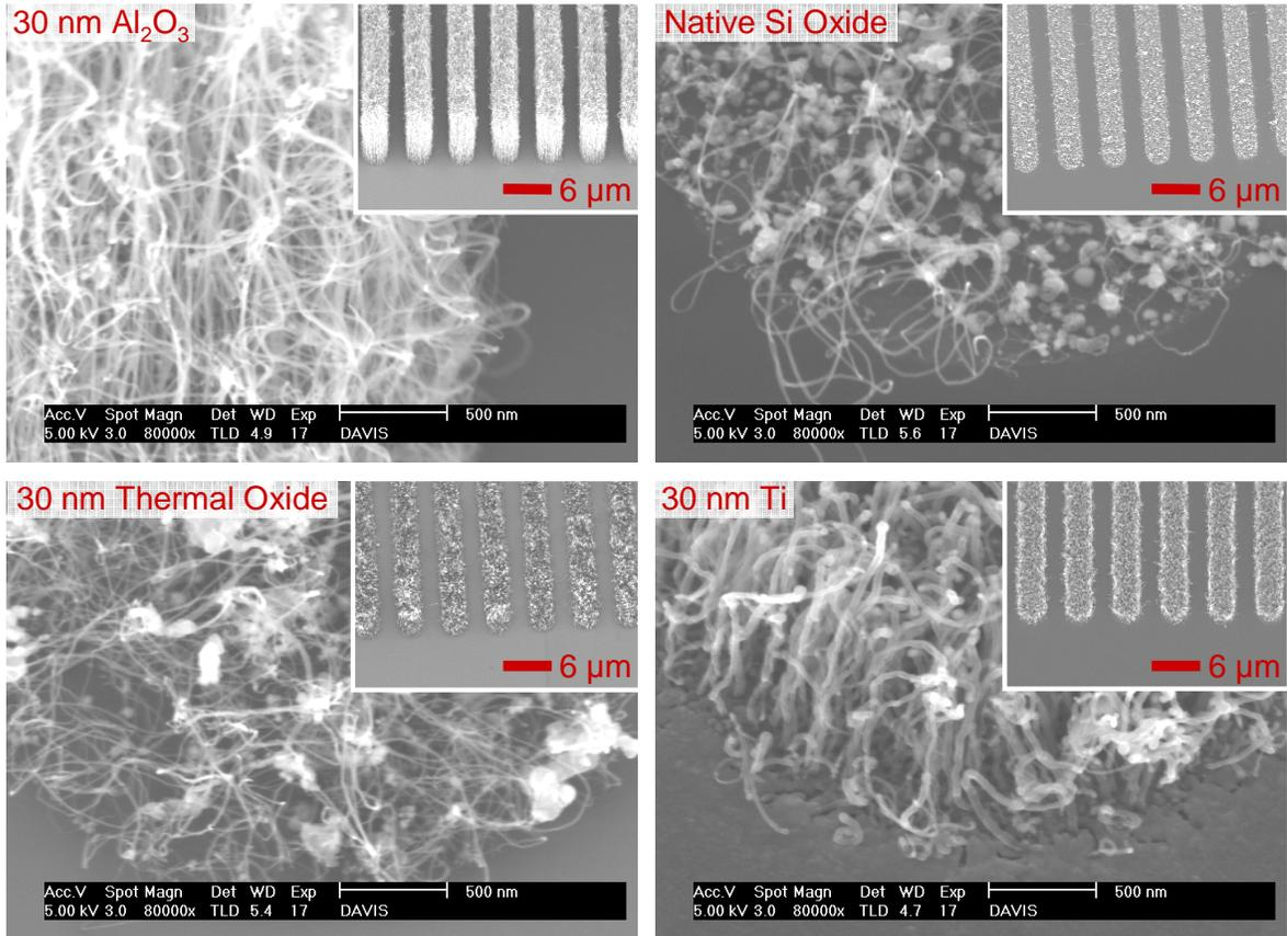
**Figure 3.1** SEM images of the VACNT forest growth with different barrier layers. Each main image shows an 80,000X image of tube density and alignment. Each inset shows a 2500X view of the VACNT structures.
