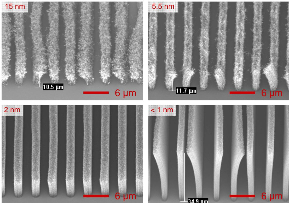
**Figure 3.5** SEM image of VACNT structures with different Fe thickness'
