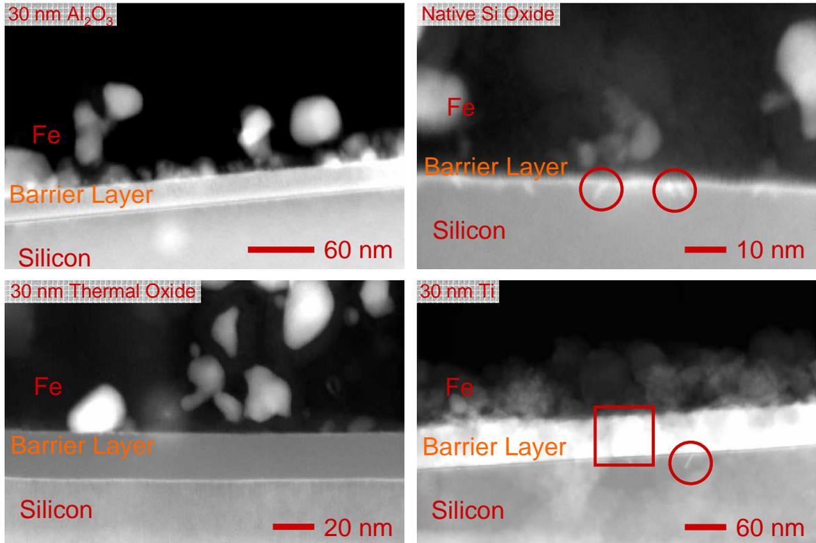
**Figure 3.2** TEM cross section of the Fe particles after growth on different barrier layers. The circles highlight Fe silicide formation and the square highlights possible alloying in the titanium.
