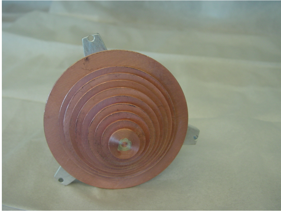
Figure 1.2: The charge collecting rings viewed from along the machine axis. Each ring corresponds to a cylindrical shell volume in the confinement system.
