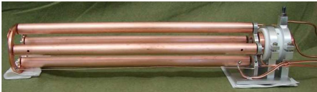
Figure D.2: The completed quadrupole. Originally, the poles and the support piece at the far left in the picture were aluminum.
