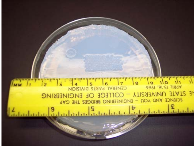
Figure 2. A 2% agarose (no Al) sample with multiple lines of laser ablation. The ring on the top left of the sample is due to the height alignment screw.
