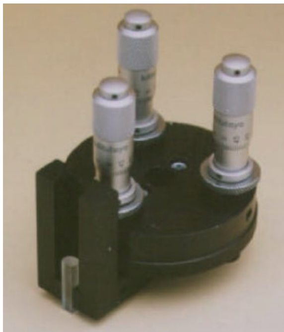
Figure 2.3 An example of a tripod used for TEM sample preparation.
