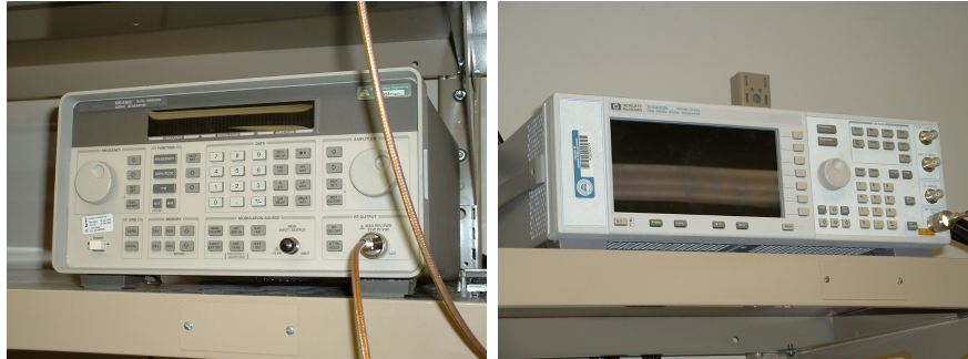
Figure 2.3: LO1 and LO2 are standard signal generators that connect to each of the RF receivers for each antenna.
