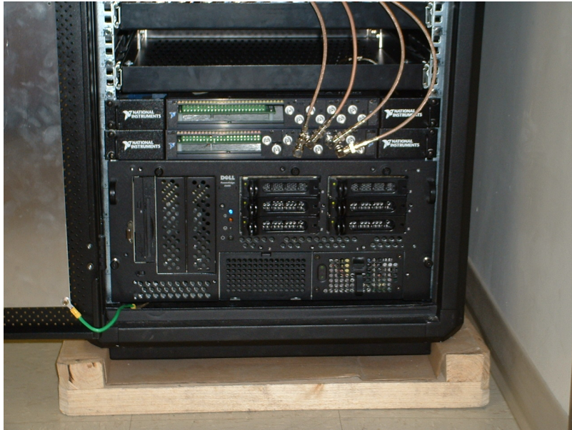
Figure 2.5: The A to D converter sits below the IF filters and amplifiers. It is the last step before the signals acquired by the radio antennas reach the computer for processing.
