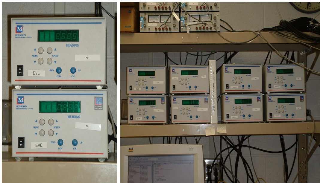
Figure 2.9: Four sets of azimuth and elevation control boxes sit beneath the power supplies and above Computer A. They are labeled with numbers and the names of each antenna: 1.) Eve, 2.) Sarah, 3.) Rebekah, and 4.) Rachel.
