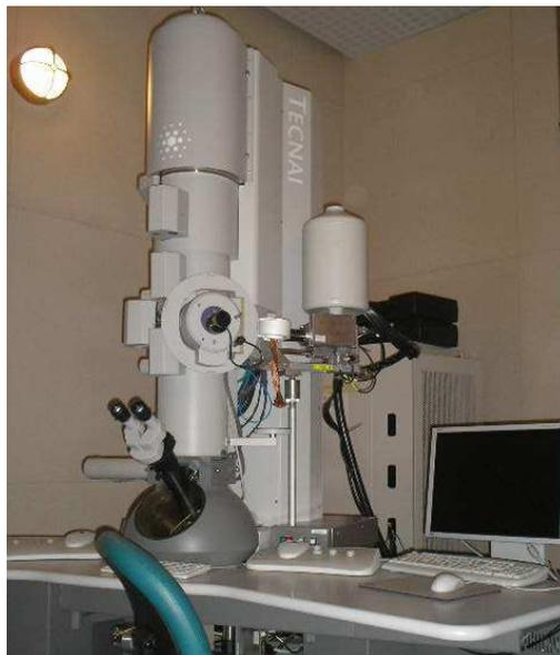
**Figure 2.1** Tecnai F-20 Analytical STEM microscope. Located in the Eyring Science Center’s underground lab on Brigham Young University’s campus in Provo, Utah.
