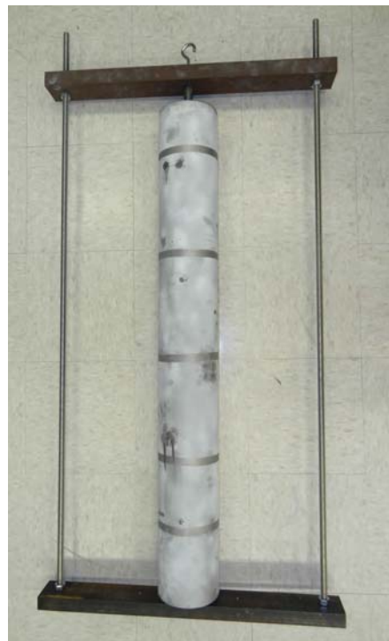
Figure 5.1 Schematic of the frame designed to hold the cylindrical shell in a fixed and stable position.
