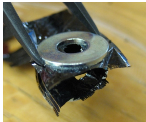
Figure 2.20 Separation of the dual layer composite from the weight of the washer it was glued to after bulge testing.
