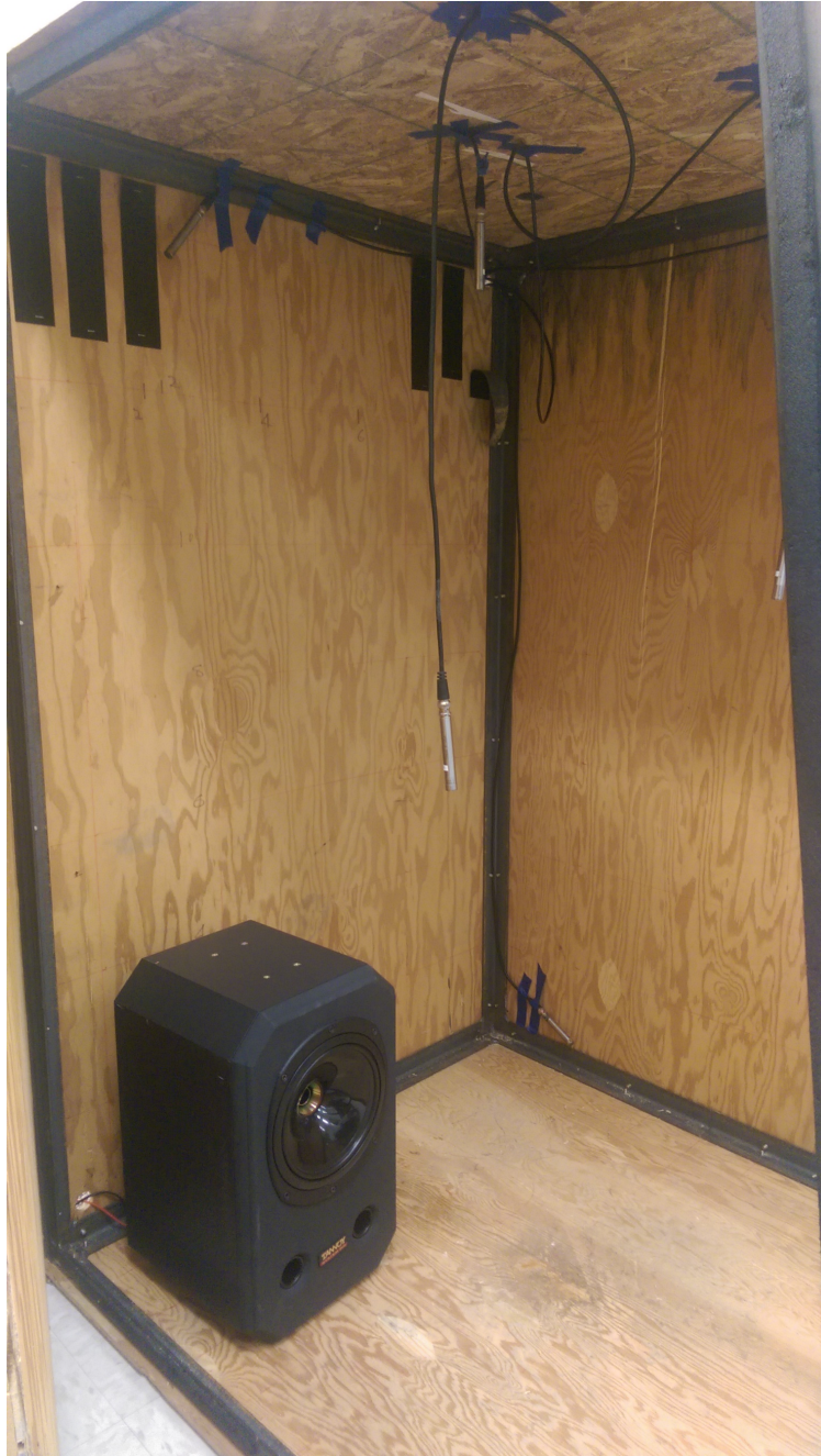
Figure 5.15 Photo of microphone and loudspeaker positions for testing 3D-printed resonator system.
