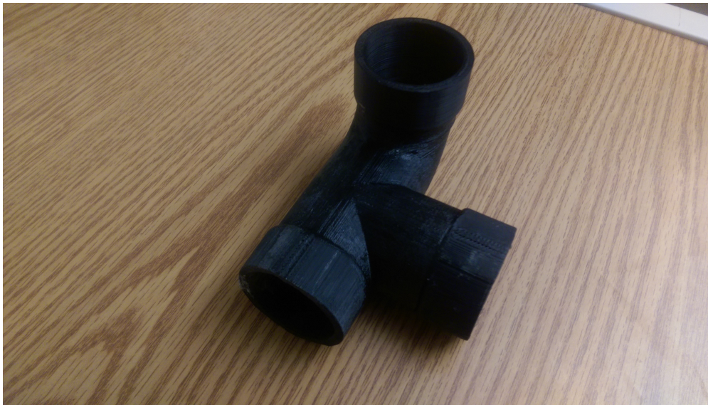
Figure 5.10 Image of 3D-printed component designed for enclosure coupling.
