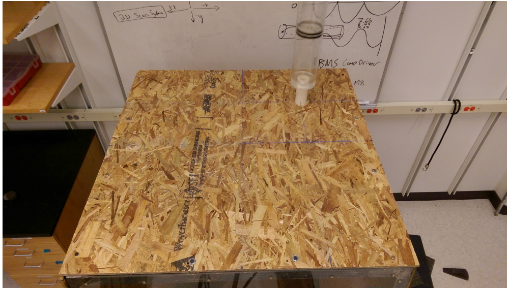
Figure 5.6 Photo of single Helmholtz resonator coupled to enclosure.
