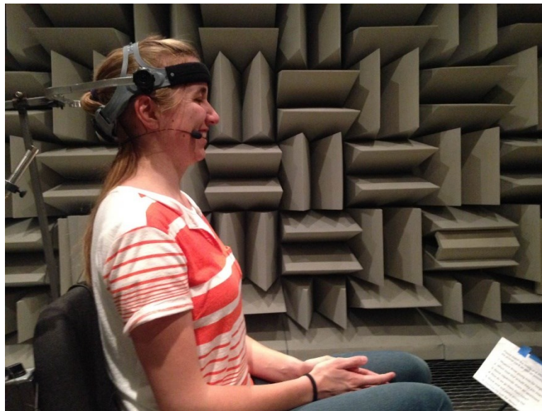
Figure 2.2. A female subject in the directivity measurement chair. The cheek-worn reference microphone, the head positioning apparatus, and the prompt paper are pictured. The earbuds used for playback are not pictured.
