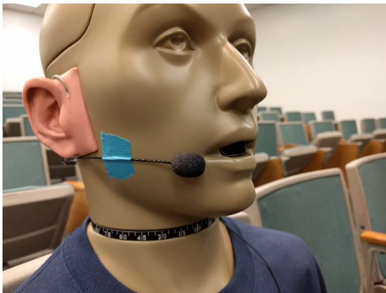
Figure 3.10. An OBRIR measurement in C215. The positioning of the head-worn microphone on KEMAR is shown.
