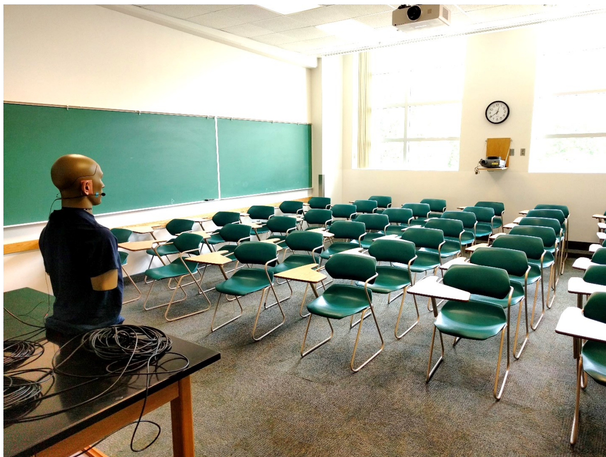
Figure 3.11. An OBRIR measurement in ESC C261. KEMAR was positioned at the front of the room, similar to where a teacher or lecturer might stand.
