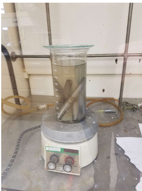
FIG. 2. Photograph of some of the samples in the hot magnesium chloride solution in a fume hood.
