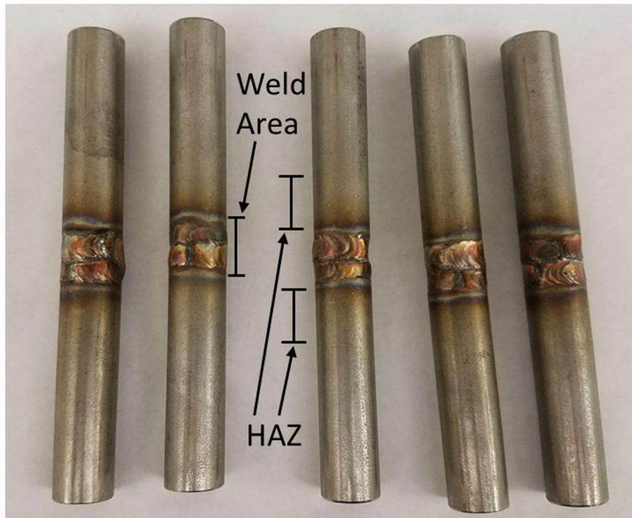
FIG. 1 Photograph of five of the samples before inducing damage. Also depicted are the weld region and the Heat Affected Zone (HAZ).
