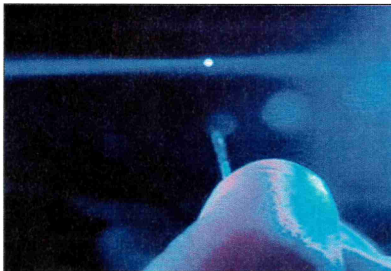
Fig 2.0.2 Method of loading. The authors thumb and sewing needle used to load the trap.
