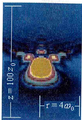
Fig 3.1.3 Spherical aberration plot. Intensity plot of a focus with spherical aberration using f# 4. The 532nm light propagates from top to bottom.
