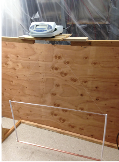
Figure 1 : A picture of our experimental setup. A digital scale is supported by a wooden frame. Suspended from the scale is the hanging testing apparatus which holds the anode and cathode parallel using an insulating PTFE frame.
