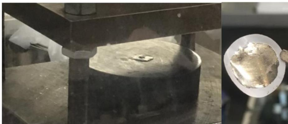
*Figure 26. Small piece of oxide-removed lithium metal foil sitting atop Celgard inside a hydraulic press (left). Lithium metal after sandwiching between two pieces of Celgard, pressing via hydraulic press, and peeling off one of the Celgard layers.*
