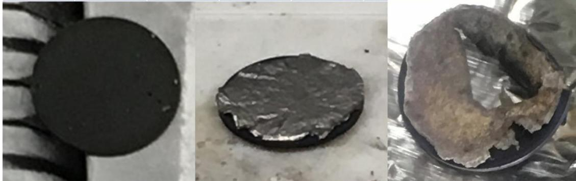
*Figure 25. Somewhat unsuccessful lithium melt infiltration into CNT forest. Various parameters associated with the experiment (top), Pre-LPCVD forest (left), molten lithium and oxides atop Si-coated forest (middle) and burned lithium atop cracked CNTs due to high temperature (right).*
