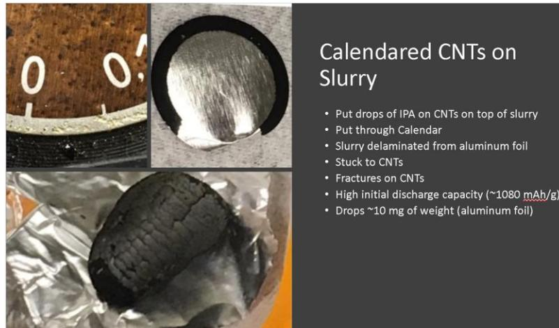
*Figure 24. Pressing CNTs and a sulfur slurry (~0.05 mm) resulted in a delaminated slurry and cracked CNTs (bottom-left). The leftover slurry and aluminum foil are shown in the (top-middle).*
