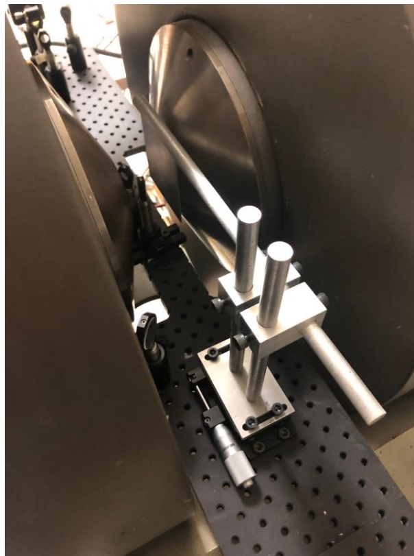
Figure 14 A picture of the actual translation device mounted on our system
