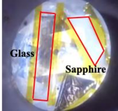
Figure 2.3. Still photo extracted from growth video during evaporation. The dark gray indicating \text{Zn}_3\text{As}_2 film growth develops on the left-hand substrate (glass) before it does on the right-hand substrate (sapphire). The amount of time from start of evaporation to darkening is highly variable from sample to sample.
