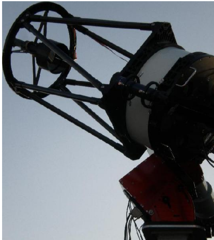
Figure 2.1 BYU's ROVOR telescope located near Delta, Utah. ROVOR was placed near Delta because of the relatively low levels of light pollution and is controlled remotely. ROVOR is a 16" (0.4 m) telescope, making it a good tool for observing bright objects. ROVOR is a member of the Whole Earth Blazar Telescope (WEBT) contributing to gathering data on blazars.
