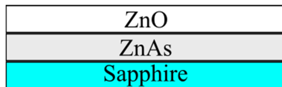
FIG. 4. Layer model. We first deposit zinc arsenide, our source of dopant, on top of our sapphire substrate. The zinc oxide is then sputtered directly onto the ZnAs layer.
