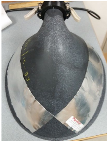
Figure 3.10: A photo of the Pyrotek constrained layer damping material applied to the bowl.
