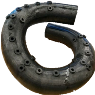
Figure 5.1: Photo of the 3D printed spiral tube with flush mounts built in.
