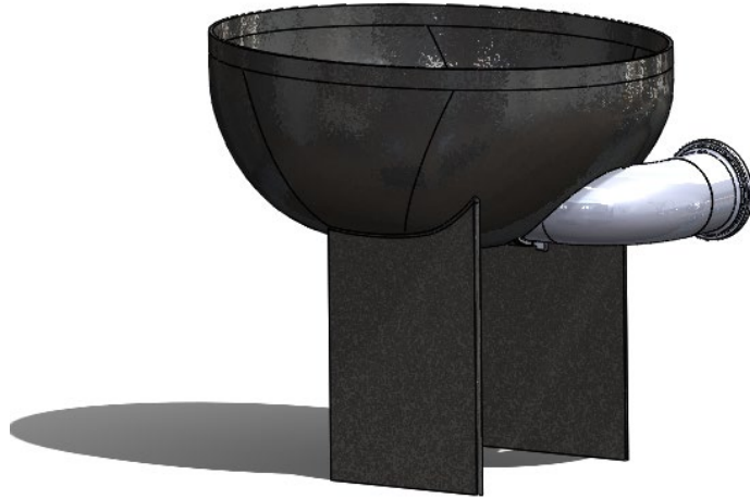
Figure 4.6: Notional diagram of baseline tube geometry in relation to the toilet
