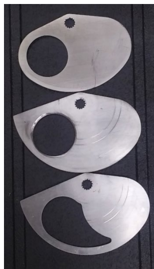
Figure 6.9: Photograph of the baseline, beveled, and shark fin valve variations
