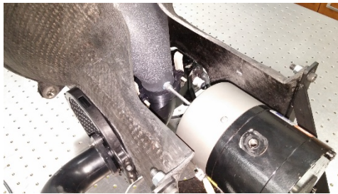
Figure 3.5: A photo of a shaker attached to the bottom of the bowl. This is where the bowl was excited for scanning laser Doppler vibrometer measurements.
