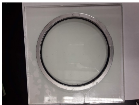
Figure 2.5 This image depicts a metal ring, silicone O-ring, and glass plate cast for the acrylic disks.
