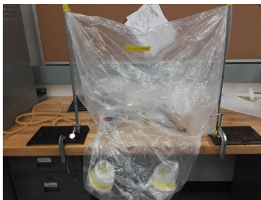
Figure 2.6 This image depicts a sealed plastic containment area filled with argon gas for the purpose of storing reactive materials.
