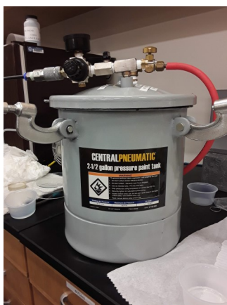
Figure 2.4 This image depicts a horizontal view of a CentralPneumatic 2-1/2 gallon pressure paint tank used to pressureize the acrylic sample and remove air bubbles.
