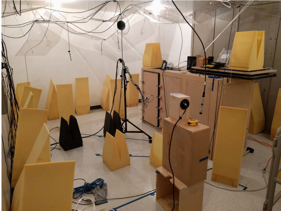
Fig 4.4. The combined sound power of three loudspeakers adjacent to the enclosure measured by the two-point method and per ISO 3741.
