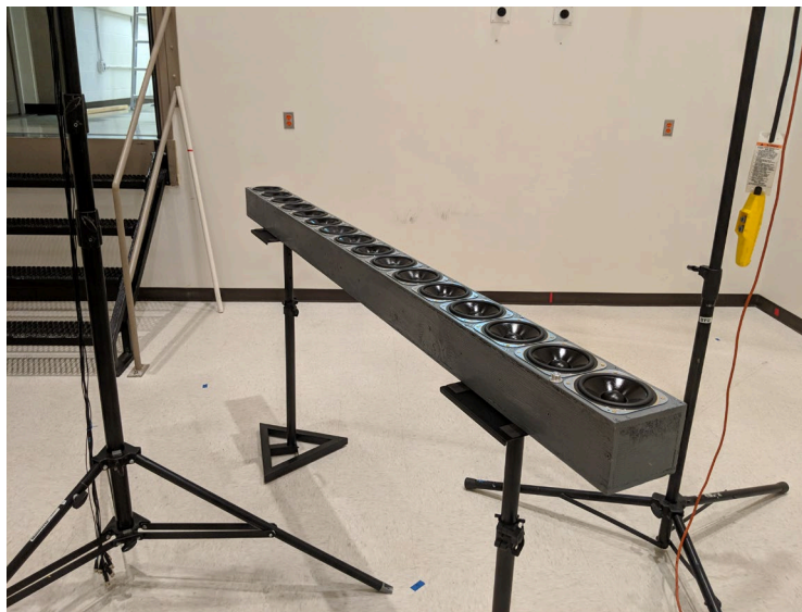
Fig 3.5. The 16-element line array pictured in the large reverberation chamber.
