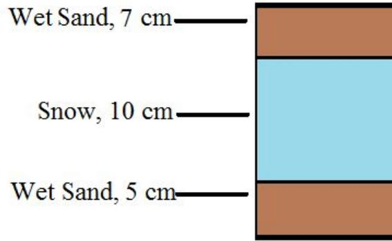
*Figure 4: Experiment 3, model with one thick layer of snow*
