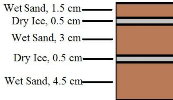
*Figure 3: Experimental Model 2, model with two thin layers of dry ice*
