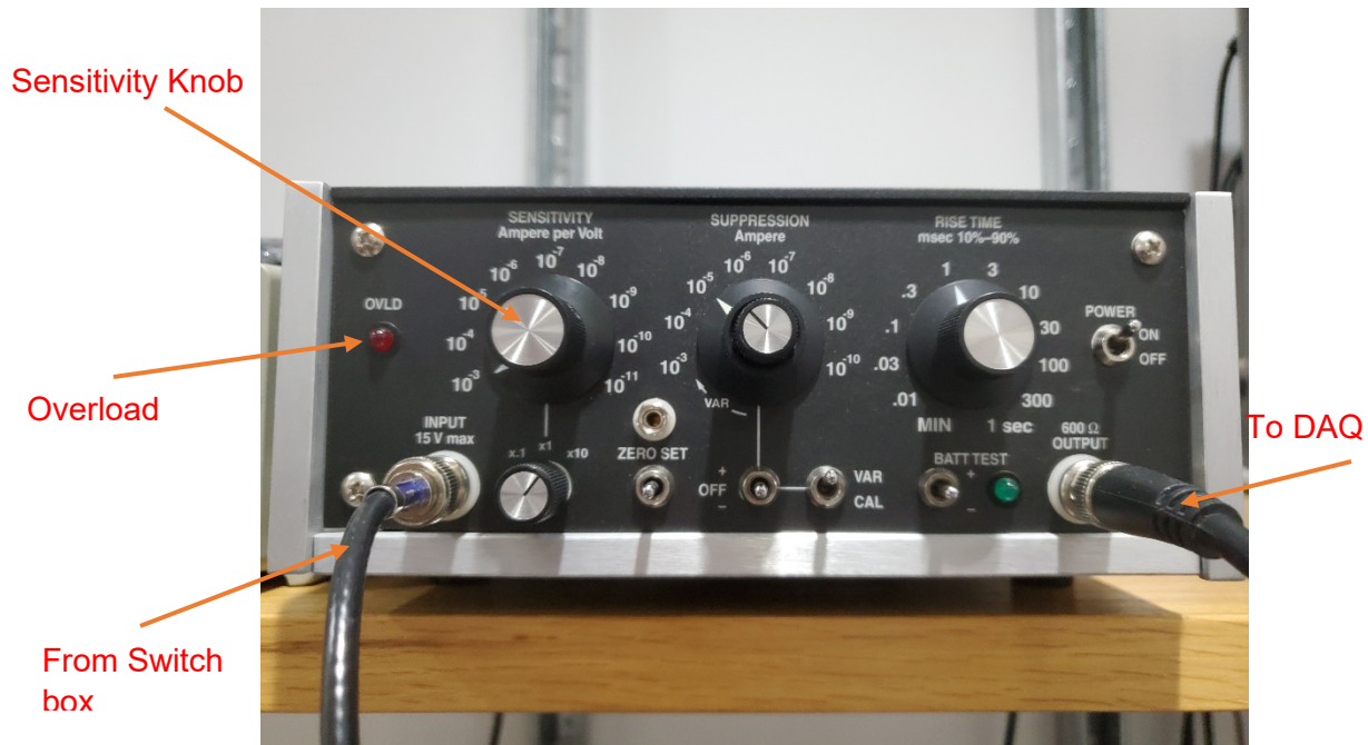
Figure 36. Preamp for four-point probe station.
