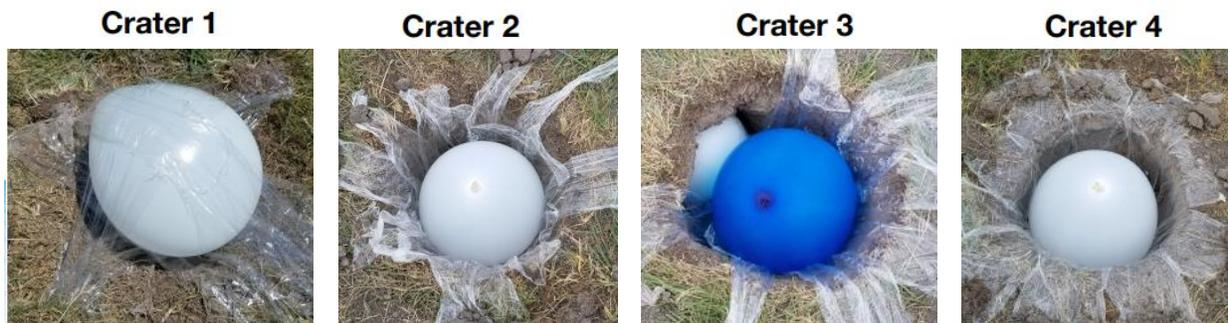
**Figure 2.5** Photograph images of each crater with the balloons placed inside. The saran wrap was used to prevent the balloons from popping prematurely.
