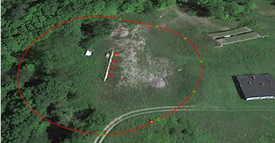
**Figure 2.2** Volcano Hazards Workshop Setup. Image of the four explosion test sites represented by the small red circles. The small green circles represent the microphone locations arranged in a semicircle around the center of the test sites.
