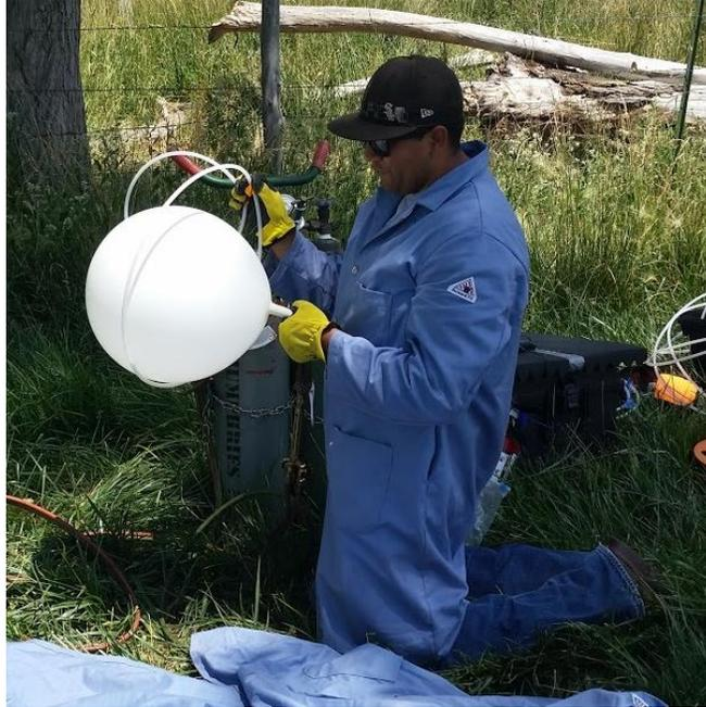
**Figure 2.3** Image showing balloons being filled. The different rings were used to fill the balloon with the proper volumes of each gas.
