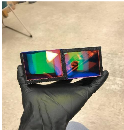
Figure 7: Picture of the final product: colorblindness goggles
