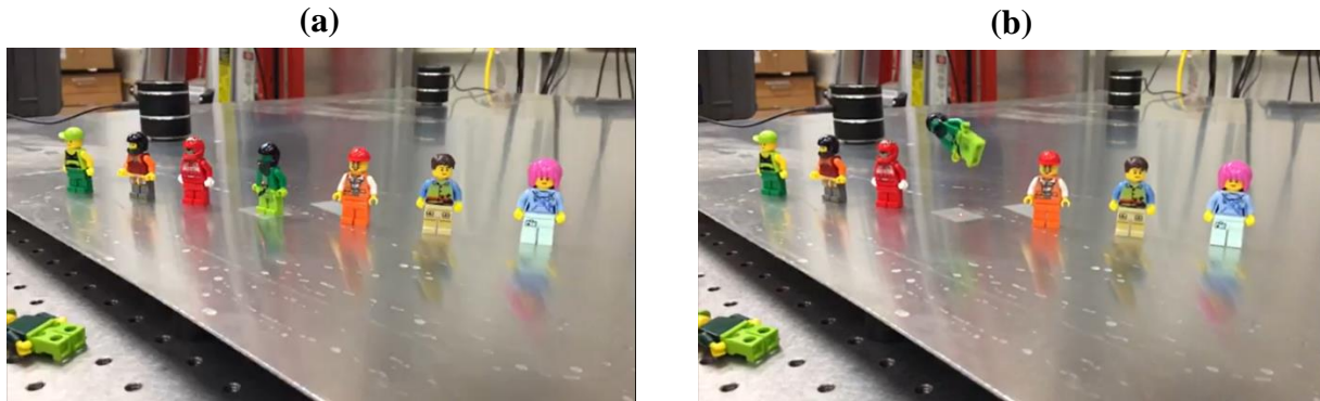
FIG. 2. (color online) (a) Setup of the LEGO demonstration with two shakers in the background and the SLDV aimed at the minifigure in the middle. (b) The airborne minifigure after the focus.
