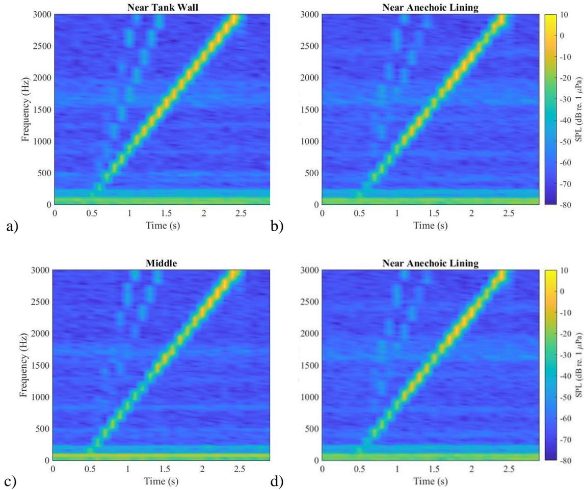
**Figure 3.1** Spectrograms of the received sound pressure level when the source-receiver pair were (a) 20 cm from tank wall, position D in Fig. 2.2(b); (b) 20 cm from anechoic lining, Fig. 2.2(b) position F; and (c) in the middle of tank, Fig. 2.2(b) position E. For convenience part (d) is a repeat of part (b).
