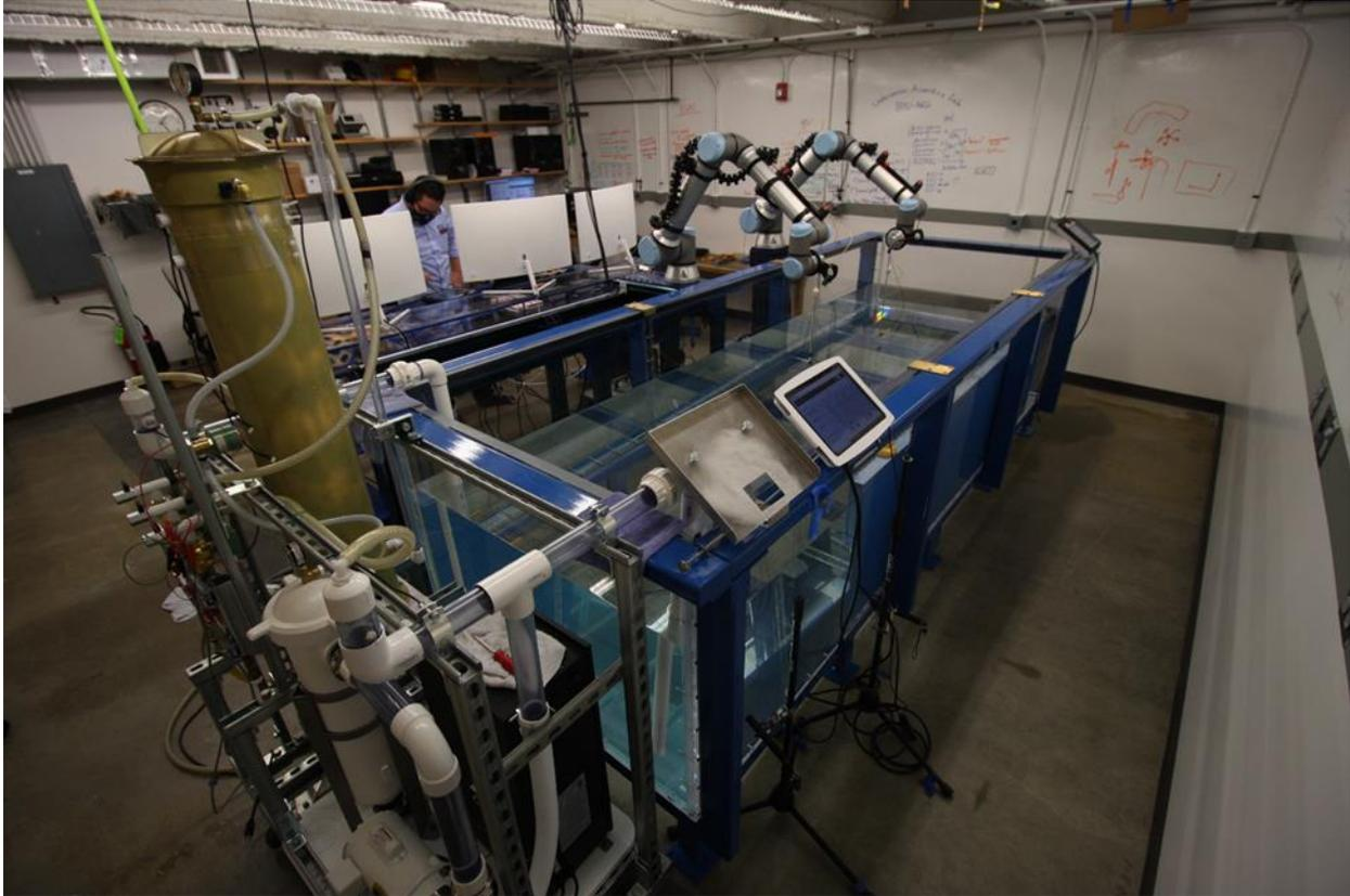
**Figure 1.3** Acrylic tank with filtration system in the Underwater Acoustics Lab at BYU
