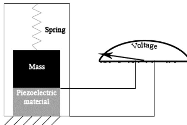
**Figure 1.1** Schematic of an accelerometer. Credit: <https://en.wikipedia.org/wiki/File:PiezoAccelTheory.gif>
