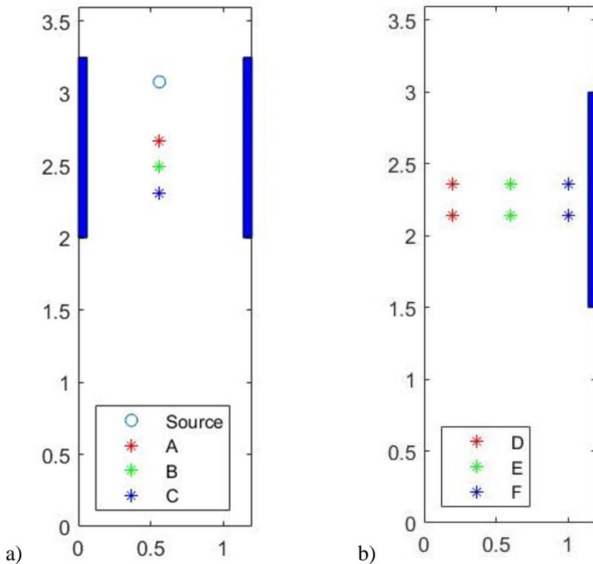
**Figure 2.2** Schematics of the 1.2 x 3.6 m acrylic tank showing the set-up of (a) the preliminary intensity measurements and (b) the anechoic panel testing. The blue rectangles designate positions of the anechoic paneling.
