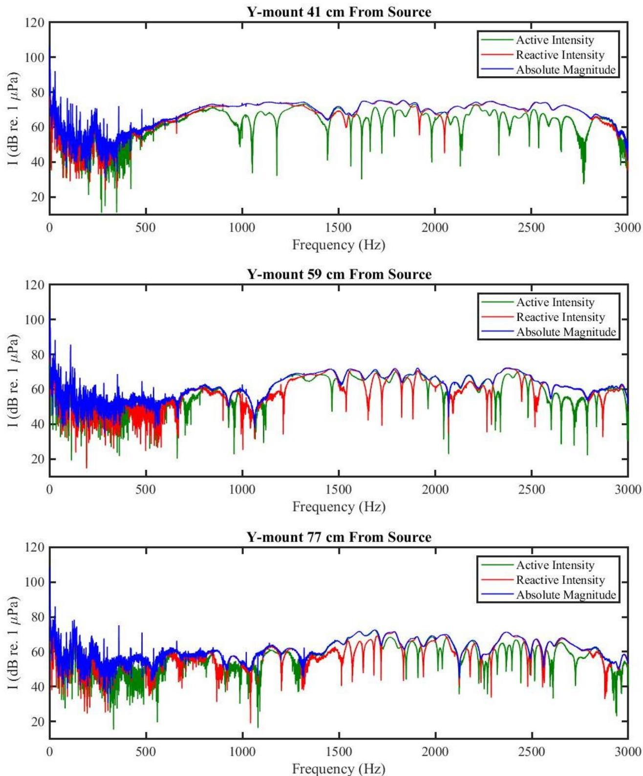
**Figure 3.4** Intensity estimates with the p-p method from two receivers on the Y-mount at different distances from source: at positions A, B, and C in Fig. 2.2(a).
