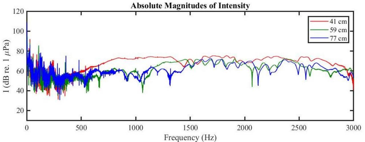
**Figure 3.5** Absolute acoustic vector intensity at various distances of receivers. The 41 cm distance line corresponds to position A in Fig. 2.2(a), the 59 cm line to position B, and the 77 cm line to position C.
