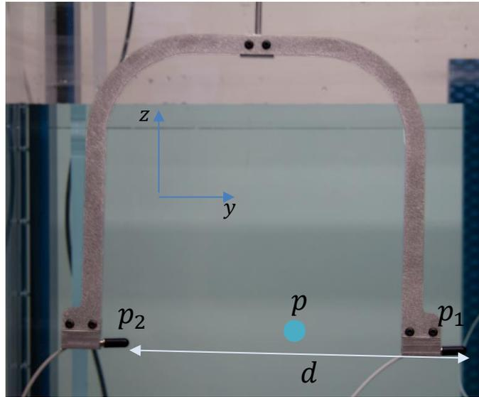
**Figure 2.1** Y-mount, a two-receiver probe, illustrating physical interpretations of above formulas.
