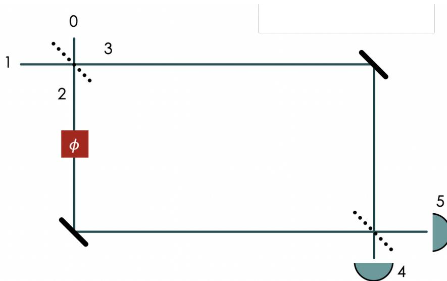
**Figure 2.2** Diagram of a Mach-Zehnder Interferometer.
