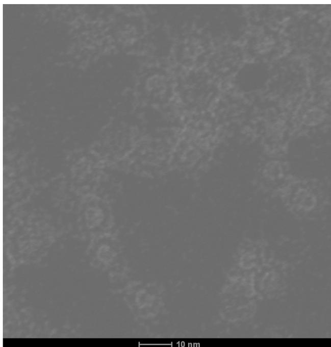
**Figure 3.3** Image of Ferritin. Note the deposition on sample causing it to lighten significantly.
