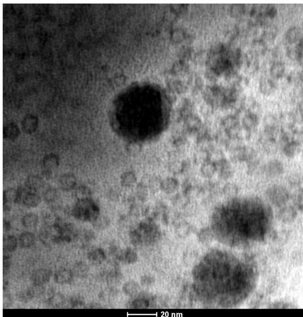
**Figure 3.1** Several ferritin molecules. Note the lack of contrast between the ferritin H and the zinc oxide core as zinc is a light metal.
