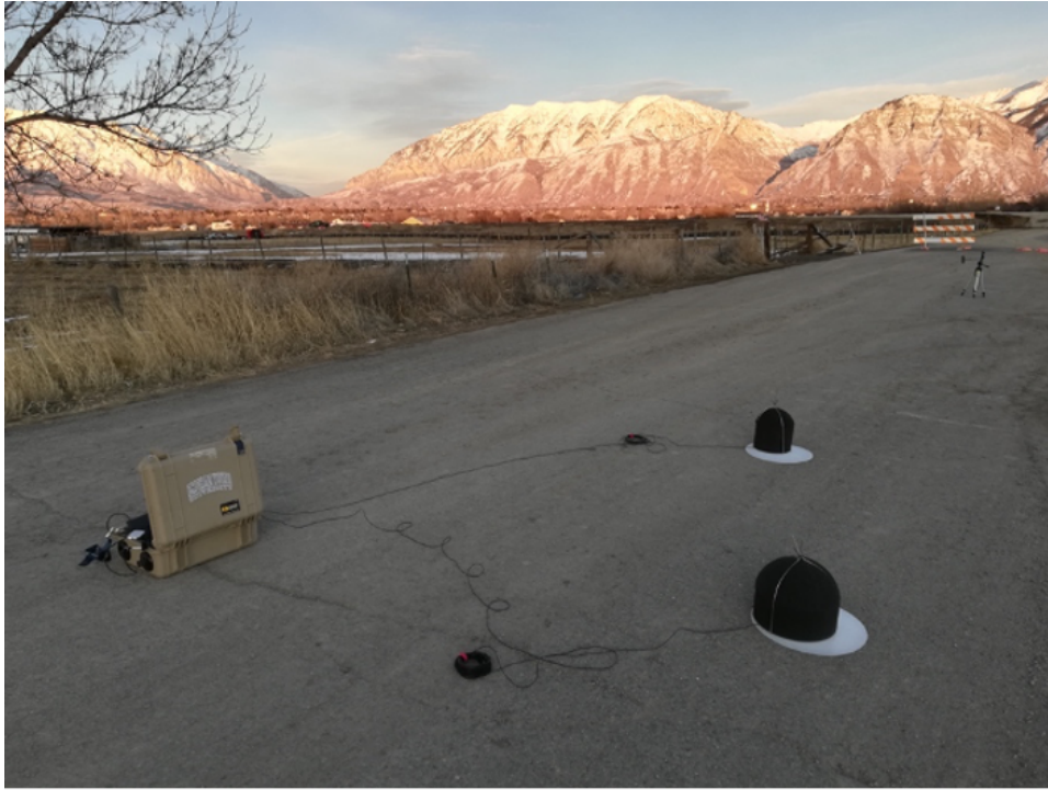
Figure 2.4 The outdoor setup used to obtain comparative wind data for COUGAR and COUGARxt. In this figure, COUGAR is shown further away from the camera and COUGARxt is closer. The wind traveled from right to left in this photograph.
