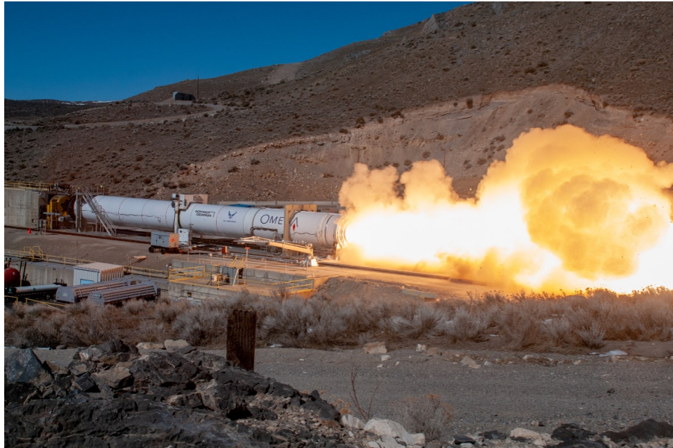
Figure 2.3 A close-up photograph of a CASTOR solid rocket motor test. The microphones were generally about 1-2 km away from the motor during testing.
