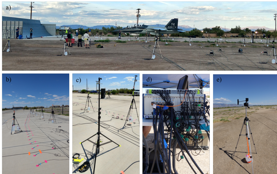
Figure 4.2 Images of T-X measurement layout at Holloman Air Force Base, New Mexico: a) tied-down aircraft with 38.1 and 19.2 m (125' and 63') arcs and maintainer mics visible, b) imaging ground array and maintainer mics facing downstream, c) 130° crackle station facing a loudspeaker located at the MARP, d) Imaging array data acquisition unit, and e) Kestrel weather station located at 57.2 m (187.5') along the 70° radial.
