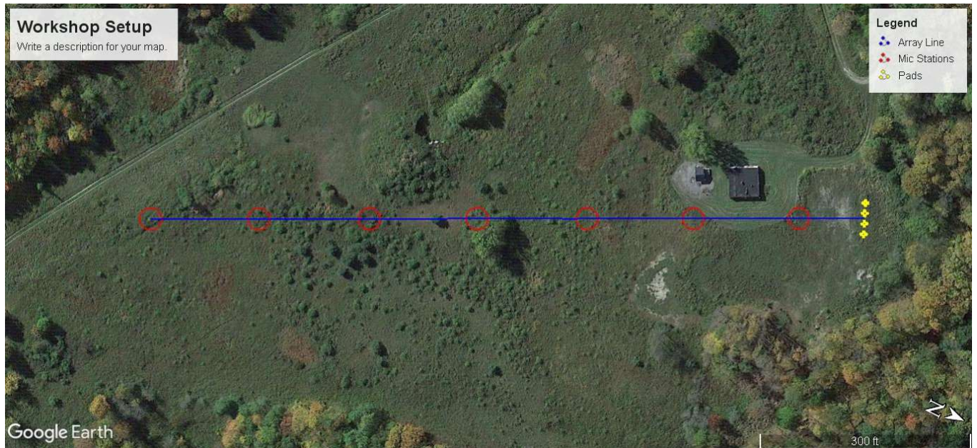
Figure 2-7 Aerial view of the set-up at the University of Buffalo Geohazards Workshop. The blast pads are marked with yellow. The array line extends out from the center of the blast pads to the last station. The array stations are marked with red circles which are placed 30 m, 80 m, 130 m, 180 m, 230 m, 280 m, and 330 m from the blast pads.
