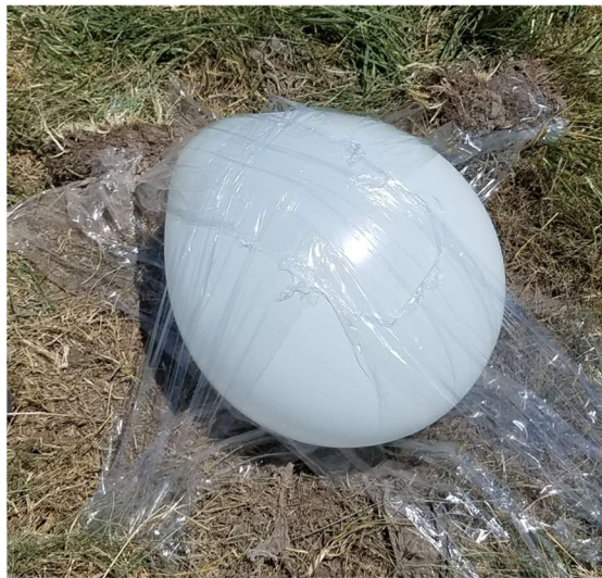
Figure 2-2 Oxyacetylene balloon held to the ground with Saran wrap to prevent popping and being blown away.
