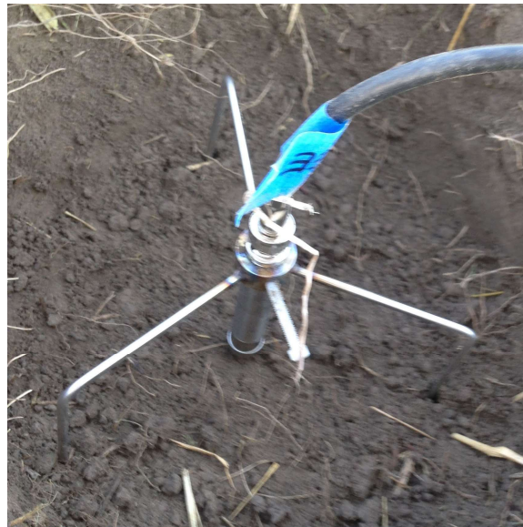
Figure 2-5 Picture of the "Ground Mic". All ground microphones were inverted on these three-pronged stands. The microphone is facing downwards with grid cap less than <math><1\text{ cm}</math> above the ground.
