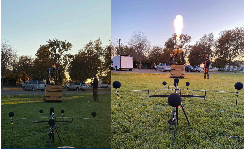
Figure 3.1.2 Experiment setup, there are two probes, both are aligned to have a zero-degree intensity direction. Left: Burner off cycle. Right: Burner on cycle.
