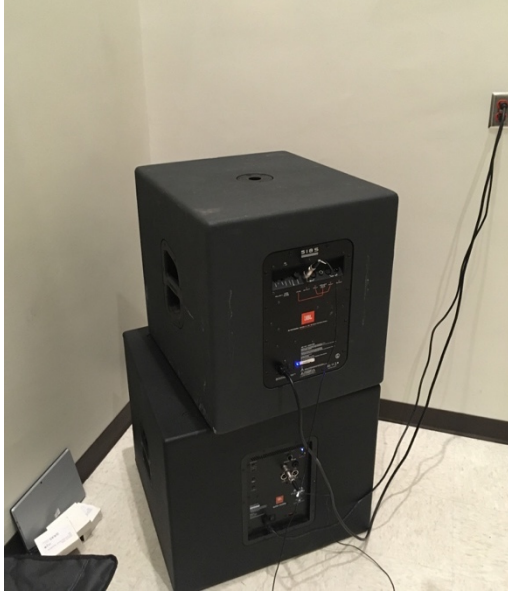
Figure 2.2.11 Reverberation chamber experiment layout. Two subwoofers were placed in the corner of the room facing against the wall. Microphones were located on the floor at the other corner of the room using the same array configuration used in the car.
