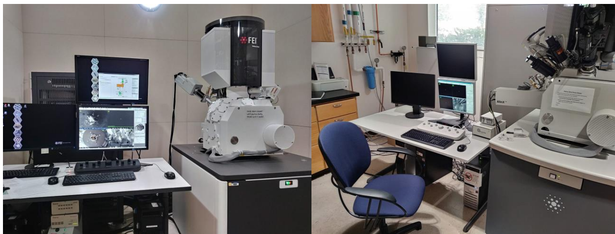
Figure 2.1 Verios SEM (left) and Helios SEM/FIB (right).
