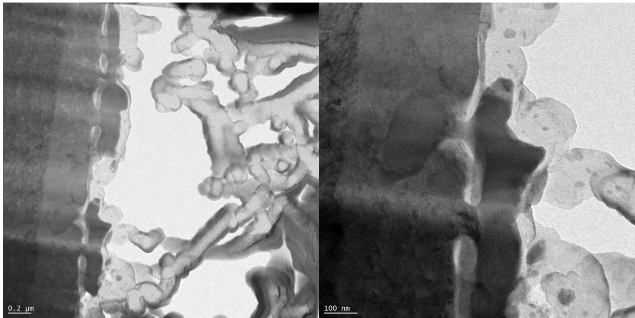
Figure 3.32 Sample 15 with TEM, showing substrate, surface layer and carbon nanotubes. The scale bars from left to right are 200, and 100 nm (respectively).
