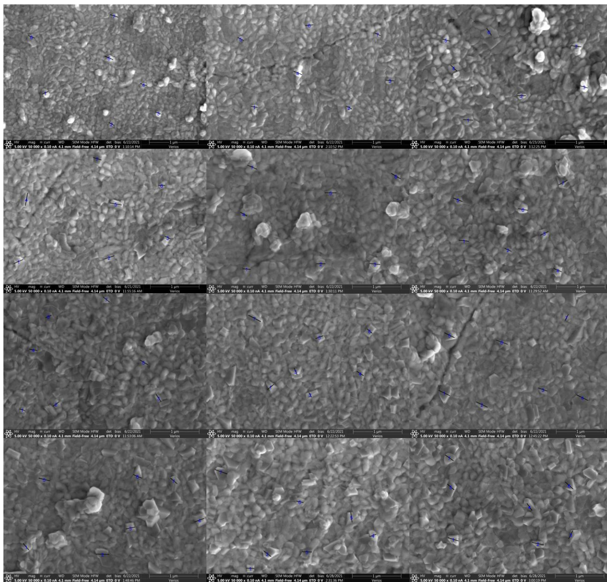
Figure 2.11 Scanning Electron Micrographs (SEM) of samples 1-12: The columns represent 1, 2, and 4 minutes in air. The rows represent 0, 5, 10, and 20 minutes in argon. A constant temperature of 800°C was kept during the air and argon flows. The scale bar for all these images is 1μm. The top right-hand corner is Sample 3, and the bottom right-hand corner is Sample 12.
