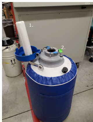
Figure 2.2 Liquid nitrogen dewar used to store samples in. 1: the neck core tube used to keep out contaminants while ensuring no pressure build up. 2: Dippers which allowed specific samples separation.
