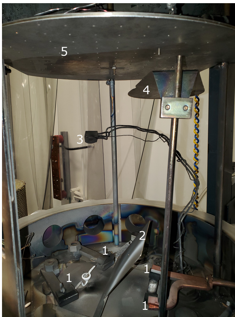
Figure 2.1 Inside of the evaporation chamber. 1: The connection points for the evaporation boats. 2: A lower shutter which can cover one evaporation boat while the other is being deposited on the substrate. 3: INFICON quartz thickness monitor. 4: The upper shutter used to control when the samples have material deposited on them. 5: the platen which samples were secured to.
