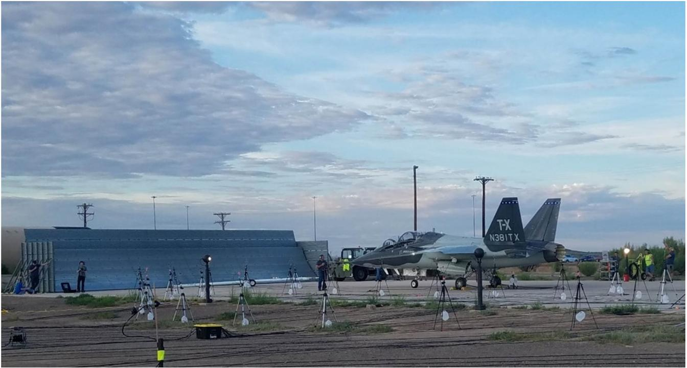
**Figure 2.1** T-7A tied to concrete pad with nose facing jet blast deflector at Holloman AFB.
