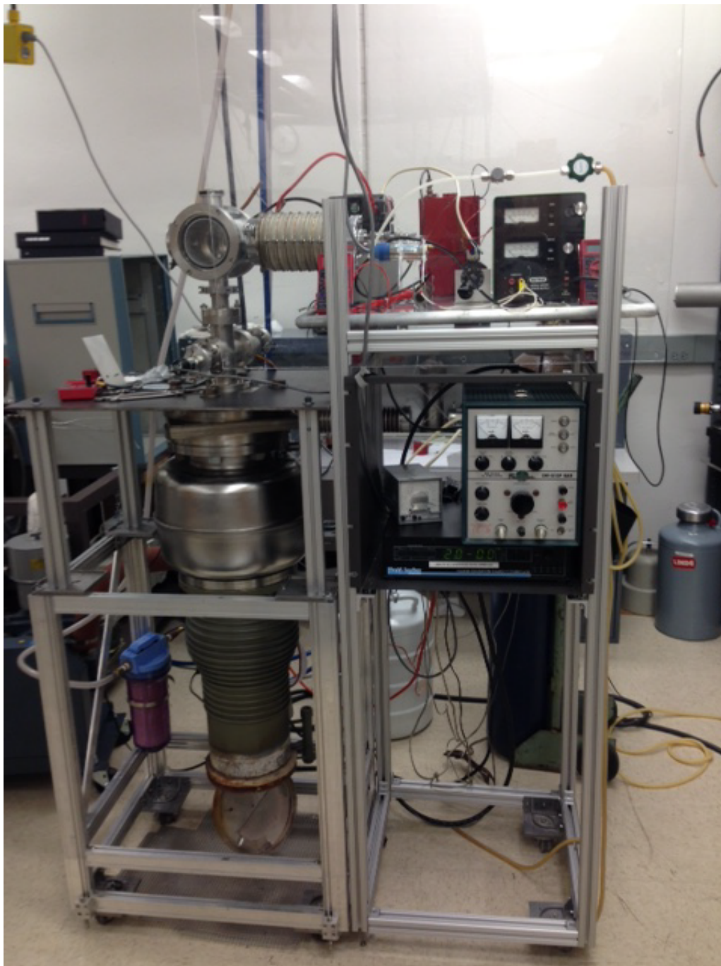
Figure 2.16 The full setup of the vacuum system, accelerator and high voltage controls.
