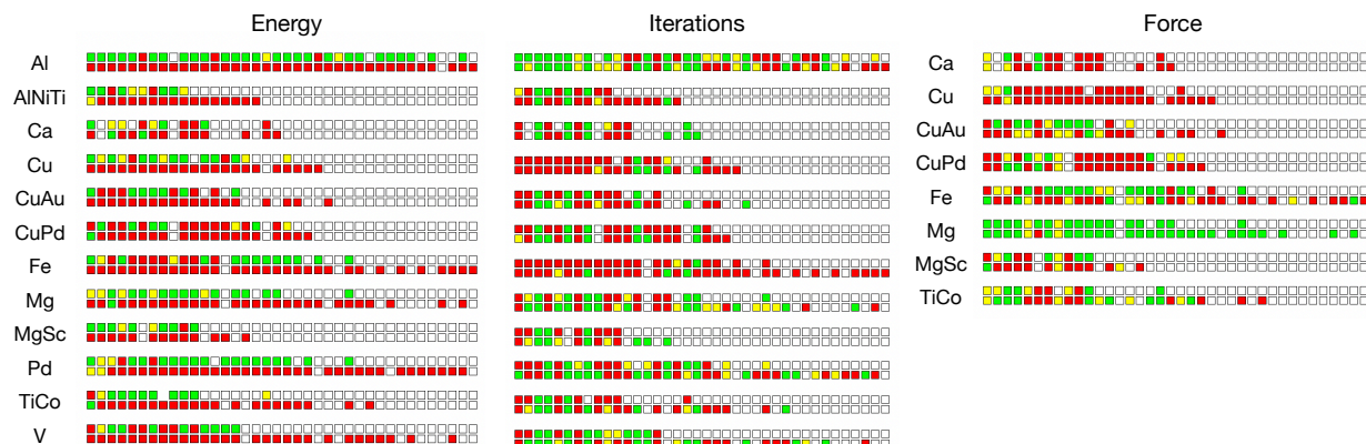
Figure 6.9 The total energies, forces and number of SCF iterations in VASP with tetrahedron methods compared against the same values obtained without smearing or tetrahedra. The tetrahedron methods down the rows are linear and Blöchl’s tetrahedra. The k -point density gets larger with each column (number of k -points is 3^3, 4^3, \dots, 40^3 ). Blöchl’s tetrahedron method most often improves the total energy accuracy. Tetrahedron methods may improve or reduce the number of SCF iterations and force accuracies, giving random and mixed results for both. Only for Mg did tetrahedra consistently improved the forces.
