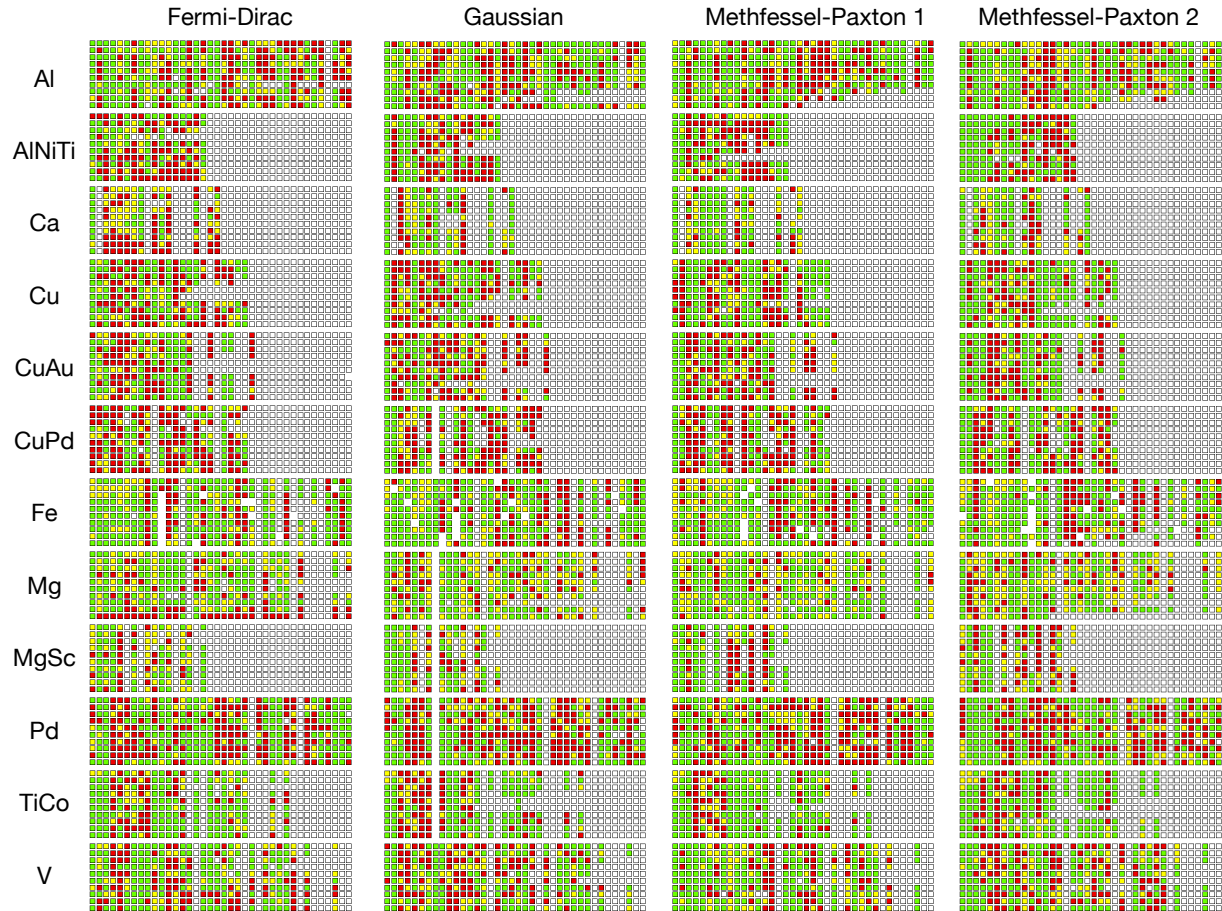
Figure 6.8 Comparison of the number of SCF iterations in VASP with and without smearing. The value of the smearing parameter increasing down the rows (value in eV are 1.0 \times 10^{-3} , 1.0 \times 10^{-2} , 2.5 \times 10^{-2} , 5.0 \times 10^{-2} , 7.5 \times 10^{-2} , 1.0 \times 10^{-1} , 2.5 \times 10^{-1} , 5.0 \times 10^{-1} , 7.5 \times 10^{-1} , and 1.0 \times 10^0 ). The k -point density gets larger with each column (number of k -points is 3^3 , 4^3 , \dots , 40^3 ). Smearing most often decreases the number of SCF iterations in VASP by at least 1 iteration; it less often but frequently increases the number of SCF iterations by 1.
