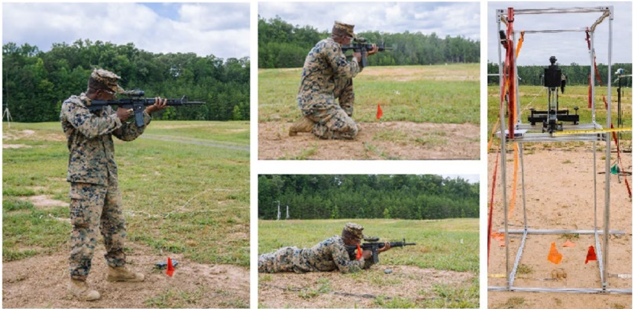
Figure 2-6. Images showing a standing, kneeling, and prone shooter. The low acoustics profile mechanical shooter stand is shown on the far right.
