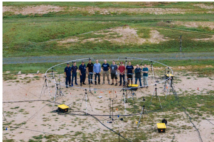
Figure 2-3 Circular arc array with measurement team standing in the middle for scale.
