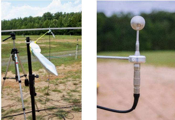
Figure 2-5. (Left) PCB 137B21B Pencil probe. (Right) Image of GRAS 3D Vector Probe.
