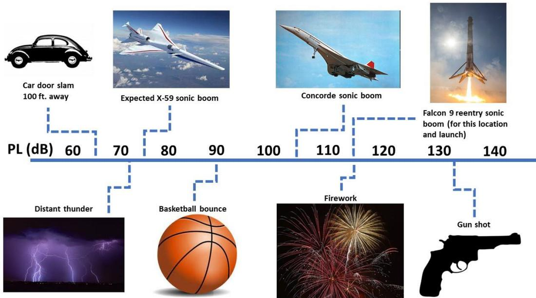
**Figure 4.** The PL values of different noise sources are compared. Three supersonic vehicles are included, with NASA's X-59 expected to be the quietest at 75 dB. The Concorde's sonic booms were much louder at 105 dB, and the Falcon 9 sonic boom for this location and launch was even louder at 115 dB. For more details of these measurements, see Ref. [18].
