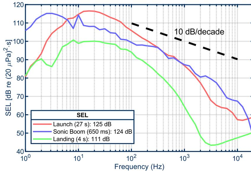
**Figure 8.** OTO spectral comparison between the launch, sonic boom, and landing noise, with the total SEL values included for each phase and time intervals used for calculation after trimming to 6 dB-down points.
