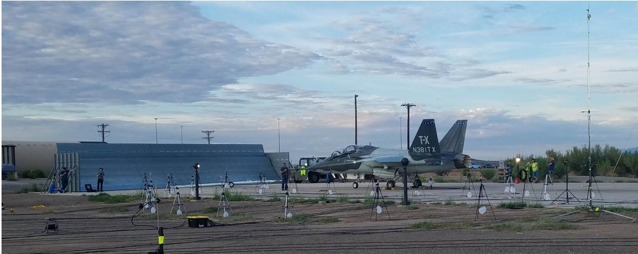
**Figure 2.1** Picture of the T-7A aircraft on the run-up pad facing the jet blast deflector. Some mounted microphone arrays can be seen in the foreground. Photo taken by a member of BYU's jet noise research group.
