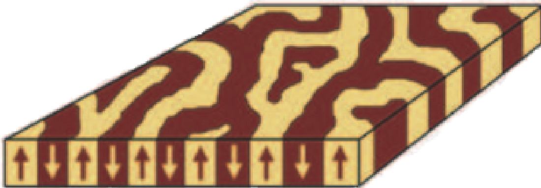
Figure 1.2 Illustration of a magnetic domain pattern with magnetization directed up and down out-of-plane.
