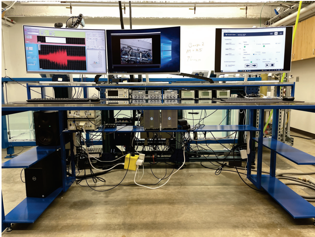
Figure 8: Computers and transducers used in the measurement chain. The ESAU interface is on the left screen; video feed from cameras in the lab are on the middle screen; and the interface for manual control of the Vention 7th axis-extender is on the right screen. Under the monitors but on top of the desk are the pre-amplifiers and signal conditioners. On the shelf below the desk, two TEGAM power amplifiers are on the left, next to the speaker, and the two chassis holding the Spectrum input and output cards are on the right.
